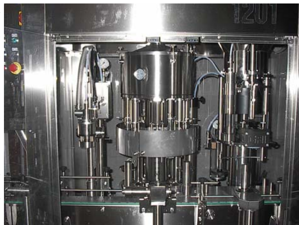
The newest component of our bottling line—A GAI Monobloc—which fills the bottles with inert gas, fill them with wine under vacuum and corks with vacuum. Top notch technology.
