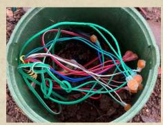
Buried in the soil are three moisture sensors and are buried at 12", 24" and 36" deep.
